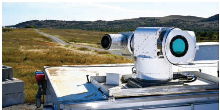
The Lockheed Martin Advanced Tactical High Energy Asset (ATHENA) is a prototype laser weapon system to defeat close-in, low-value threats such as improvised rockets, unmanned aerial systems, land vehicles, and small boats.
