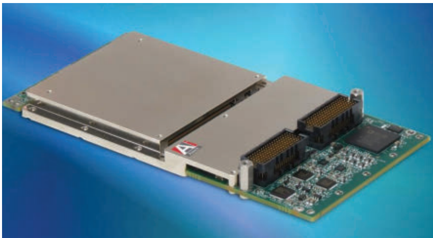
The Aitech M599 graphics embedded computing switched mezzanine card (XMC) is for mission-critical applications that call for real-time operating systems (RTOS).
