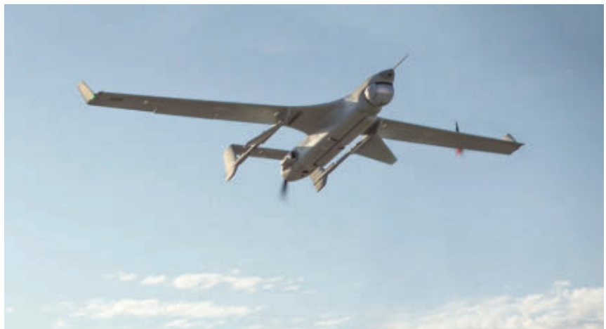
The multi-mission RQ-21A Blackjack's open-architecture payload bays can be customized with visible-light and infrared cameras, communications, and other tools.
