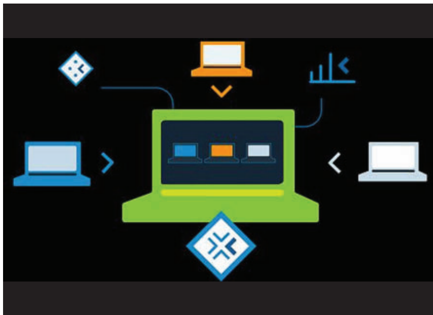
The Helix Virtualization Platform from Wind River Systems is a software-development tool based on a certifiable Type-1 hypervisor that enables applications with different levels of criticality to run simultaneously on one multi-core system.
